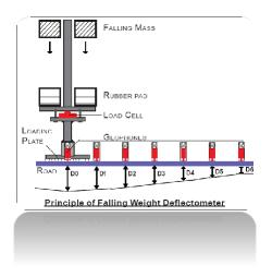
**GEOAXIS FWD** is fully automated and requires only **one man operation**. In in-built model vehicle need not be running for measuring pavement deflections, necessary power is supplied by battery provided with FWD. The unit is provided with user friendly **window based software** for data analysis and parameter calculations.
